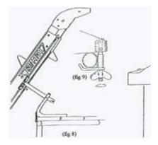
**H** With the machine secured at the scaffold the delivery shute is now fitted by slotting in the shute to the head lugs, then rotating to the required angle, extended and fixed (fig 10).
