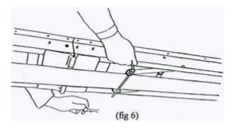
**F** The machine can now be raised to the roof/scaffold either by rope or by walking the head up a ladder. The base is guided and positioned by man 1.
