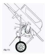
3. Rotate engine belt tensioner (fig 14) into place and operate lever to tension belts rotate belt, guard back up and lock fastener (fig 13).
